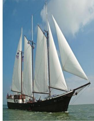
Technical data: MARE FAN FRYSLAN a three-mast schooner. Length over all 62 m. Width 7.20 m. Draft 1.50 m. Surface area of the sails - 650 m<sup>2</sup>. Passenger capacity - 27 to 40. A crew of 3-4 persons.
